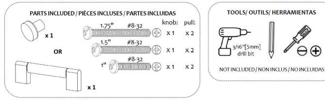
**MOUNTING INSTRUCTIONS:** This knob/Pull includes hardware that is designed to mount securely to drawer-fronts or cabinet doors that have a thickness range between 1/2" and 1-1/2" inches. If you drawer-front or door is thicker or thinner than this range, please obtain the appropriate size screw from your local hardware store.
