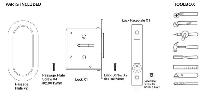
Door Thickness: This item is designed to work with pocket doors of 1-3/8" thickness.
