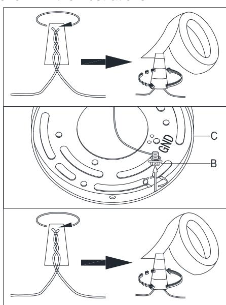
Connect the GROUND FIXTURE WIRE to the GROUND J-BOX WIRE (usually green insulation of bare wire) using the Plastic Wire Nut Connector (A) and wrap the connection with electrical tape. Be sure that no wire strands are exposed.
