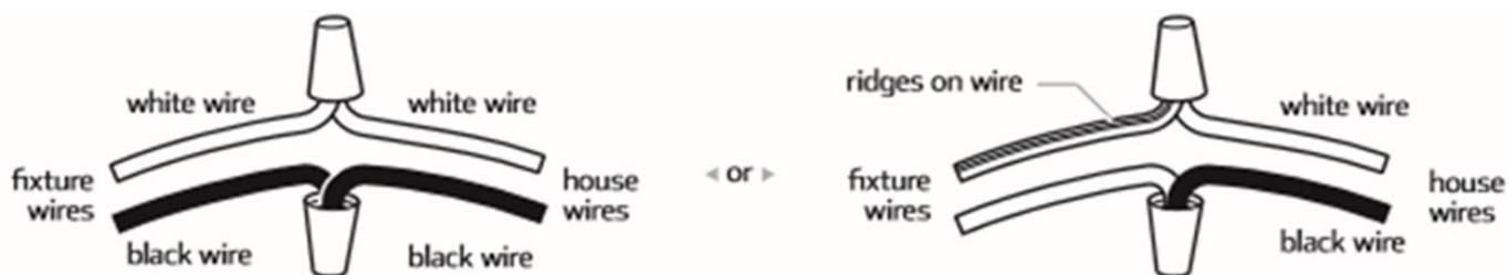
3. Carefully inspect the fixture wires. The NEUTRAL FIXTURE WIRE is White. The HOT FIXTURE WIRE is Black, and the GROUND WIRE is Bare. If you have any doubt and cannot identify the power-supply wires with confidence, then we recommend that you ask an electrician and that you not continue with the installation.
