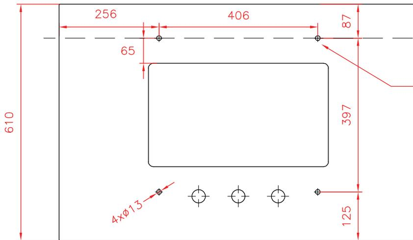
M6 FEMALE THREADED INSERT TO BE PERMANENTLY ATTACHED TOP HOLE (4 PCS).
