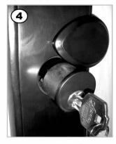
Insert the cylinder housing with the tail piece in the vertical position and then guide the tail piece and mounting posts through the deadbolt body.
