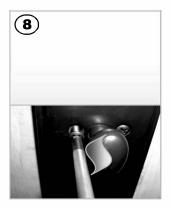
Use 1.7/16" cone-point screws to secure cylinder housing, Use of drafting or similar low tack tape will prevent marking thumb piece when tightening cylinder fixing screws.
