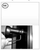
With the Allen Key supplied check the tightness of the set screw located on underside of inside lever. Fully tighten as necessary.
