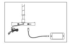
Note: There is a USB port on the fixture base, which can be used for charging USB devices (USB charging cable is not included.) The output maximum is 5V/2A. Do not overcharge.
