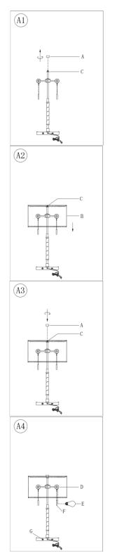
Unscrew the Final (A) from the top of Holder (C).
