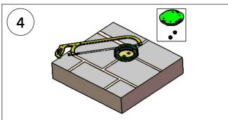
Remove the cover and outlet plugs. Cut off the excess portion of the built-in part.
