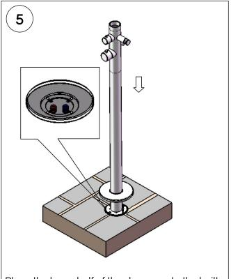
Place the lower half of the shower onto the builtin part and secure into place with (4) screws.
