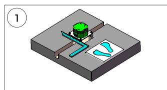
Place the built-in part in the desired position. Mark and drill the (4) holes.
