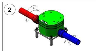
Connect the hot and cold supply pipes to the built-in part and test for any leaks.
