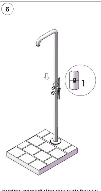
Insert the upper half of the shower into the lower half. Align and secure the screw on the back side of the shower.
