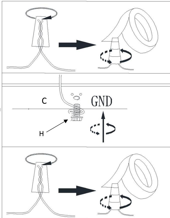
Connect the GROUND FIXTURE WIRE to the GROUND J-BOX WIRE (usually green insulation or bare wire) using the Plastic Wire Nut Connector (D) and wrap the connection with electrical tape. Be sure that no wire strands are exposed.
