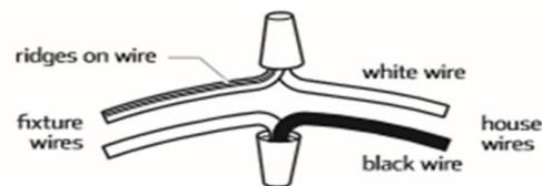
3. Carefully inspect the fixtures wires. The NEUTRAL FIXTURE WIRE is White. The HOT FIXTURE WIRE is Black. If you have any doubt and cannot identify the power-supply wires with confidence, then we recommend that you ask an electrician and that you not continue with the installation.
