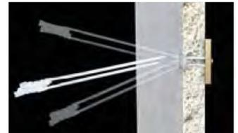
1. Slide metal channel into the pre-drilled hole
