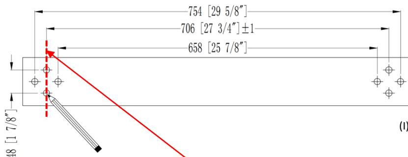
Mark on ceiling for ceiling joist location
