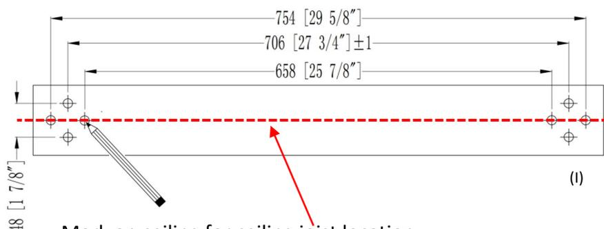
Mark on ceiling for ceiling joist location
