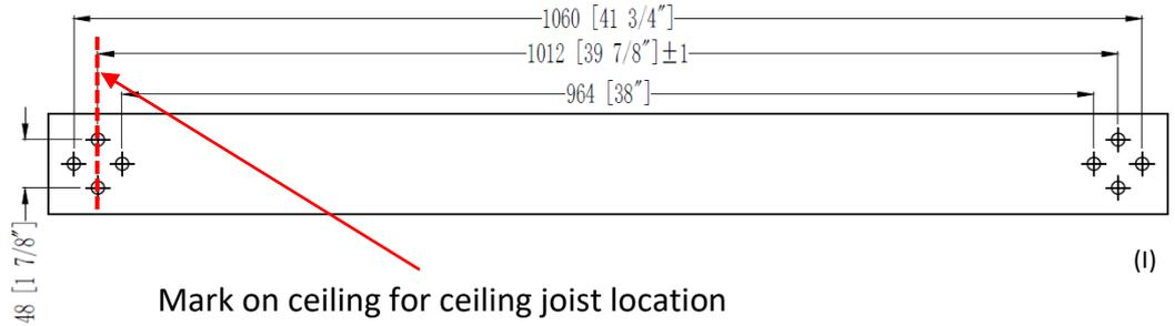
Mark on ceiling for ceiling joist location
