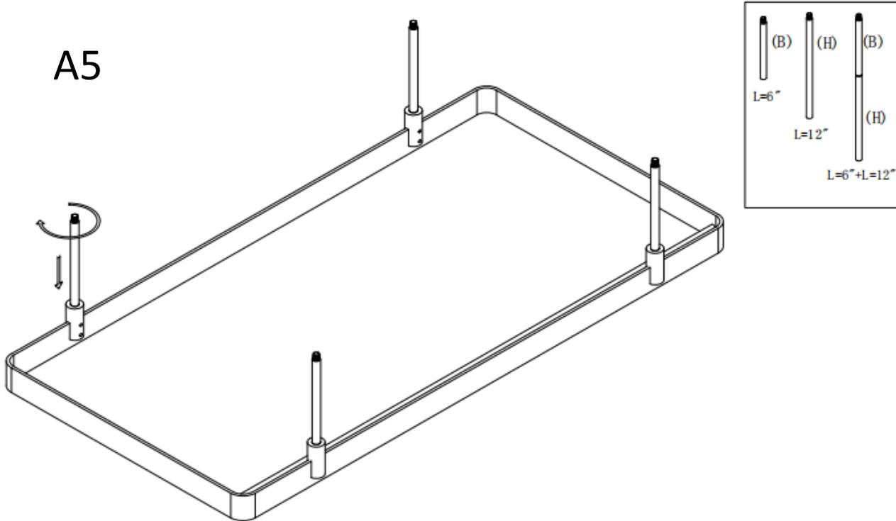
A6: Firmly tighten the flange (A) to the rod (B or H or B+H).
