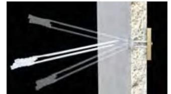
4. Push straps side to side, snapping off straps level with wall, then discard straps
