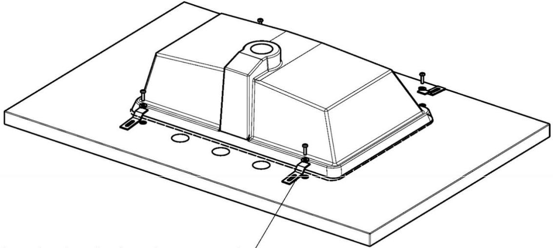
Realign sink and install 4 clips with screws per sink.
