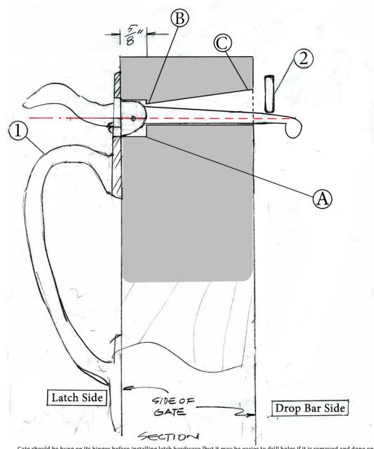
Gate should be hung on its hinges before installing latch hardware [but it may be easier to drill holes if it is removed and done on a work bench]. There should be between a ¼" and 1/8" vertical clearance gap between the gate and its post or frame.
