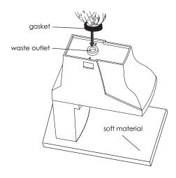
4. Holding the toilet up (2 people are recommended), align the toilet over the flange, slide the T# screws to align with the installation holes in the toilet base. Then seat the product down and press firmly until it's flat on the floor and the sealing gasket is engaged. If the toilet is lifted again, the wax ring must be replaced with a new one to ensure a proper seal.
