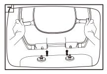
Press the buttons to lift to remove the toilet seat. Make any necessary adjustments.
