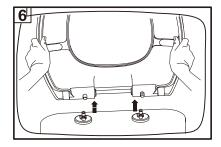
Insert the toilet seat fully into the anchors to test the alignment and operation.
