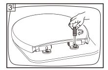
Tighten the screws until the hinges are nearly fixed, then adjust them to align with the shafts in the seat. If there is no access from the bottom of the toilet to hold the nuts, lift the hinge screw up to engage the expandable anchors to keep the nuts from spinning while securing the screw.
