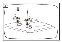
Assemble the hinges as shown and thread up the nuts to the bottom of expandable plastic anchors to prevent them from falling off, then insert the assemblies into the toilet deck holes.
