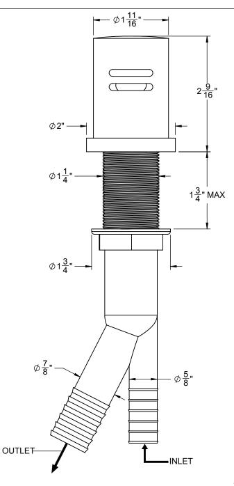
THROUGH-HOLE SPECIFICATIONS RECOMENDED MAX Ø1-1/4" Ø 1-3/8" Ø 1-9/16"
