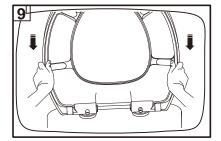
Mount the toilet seat. Make sure the hinges are fully inserted into the holes in the seat.
