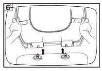
Insert the toilet seat fully into the anchors to test the alignment and operation.
