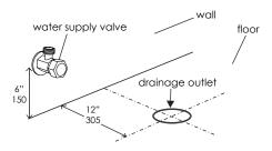
2. Align the flange with the drainage outlet and mark the location of the screws, drill pilot holes, insert anchors. Then, after inserting the two T# screws from the bottom of the flange into their position, attach the flange onto the floor over the drainage outlet.
