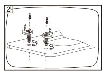
Assemble the hinges as shown and thread up the nuts to the bottom of expandable plastic anchors to prevent them from falling off, then insert the assemblies into the toilet deck holes.
