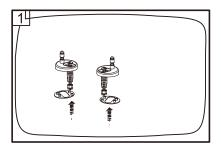
Put the clear plastic washers on the underside of preassembled seat hinges - make sure they align properly and prongs are inserted into the holes.
