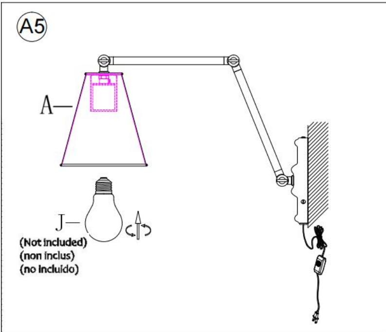
**B. Installed as a fixed mounted luminaire (hardwired assembly instruction):**
