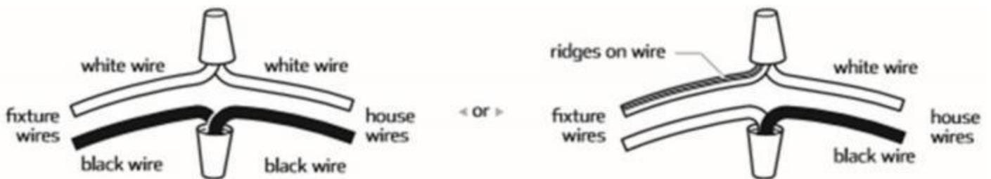
3. Carefully inspect the fixtures wires. The NEUTRAL FIXTURE WIRE is White. The HOT FIXTURE WIRE is Black. If you have any doubt and cannot identify the power-supply wires with confidence, then we recommend that you ask an electrician and that you not continue with the installation.
