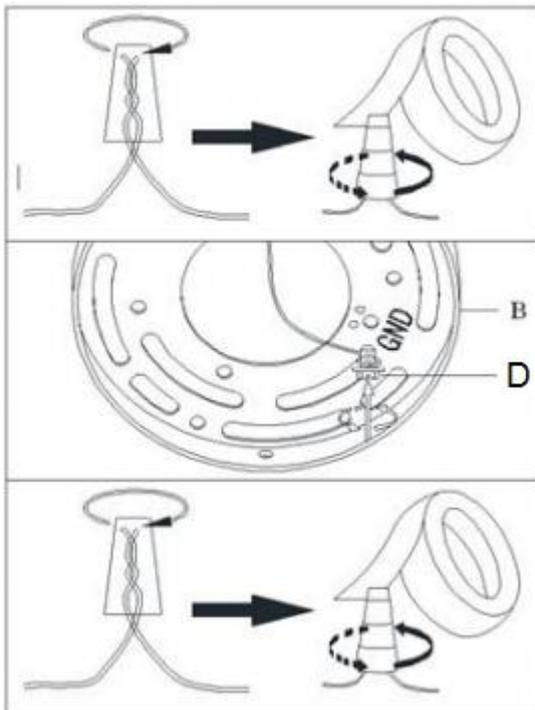
Connect the GROUND FIXTURE WIRE to the GROUND J-BOX WIRE (usually green insulation of bare wire) using the Plastic Wire Nut Connector (I) and wrap the connection with electrical tape. Be sure that no wire strands are exposed.
