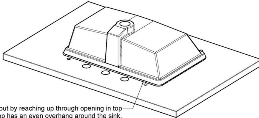
Center sink on cutout by reaching up through opening in top and verifying top has an even overhang around the sink. Once centered, mark location.
